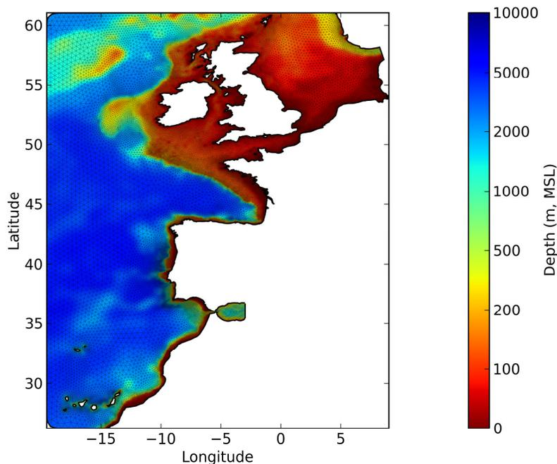
**Fig. 1. Finite element grid and bathymetry.**
