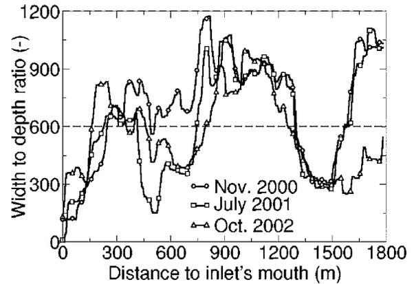
**Fig. 3.** Application of the empirical model of Allersma (1994) to three bathymetries of the Óbidos Lagoon, which relates the ratio between the channel width and the average depth to the number of channels. The number of channels should be 1 when the ratio is below 600 and 2 when the ratio is between 600 and 1,200.
