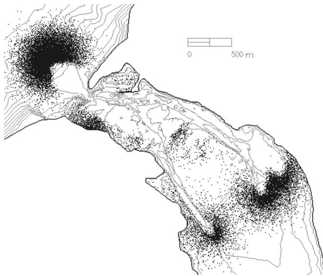
**Fig. 4.** Simulation of the fate of sand particles released in the beginning of flood at the mouth of the inlet. Each dot represents the settling location of a particle.
