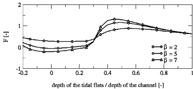
**Fig. 5.** Application of the analytical model of Fortunato and Oliveira (2005) to optimize the depth of the tidal flats. Parameter  $\beta$  represents the ratio between the width of the tidal flats and the width of the channel.  $F = \Delta t_{ef}(gh)^{0.5}/L$  represents the dimensionless rate of deformation of the tidal wave, where  $\Delta t_{ef}$  = difference between ebb and flood durations;  $g$  = gravity;  $h$  = channel depth; and  $L$  = its length.
