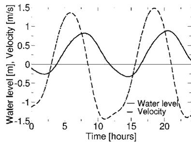
**Fig. 9.** Computed water level and east–west velocity close to the inlet mouth. On average, water levels are 60 cm higher at maximum flood than at maximum ebb.
