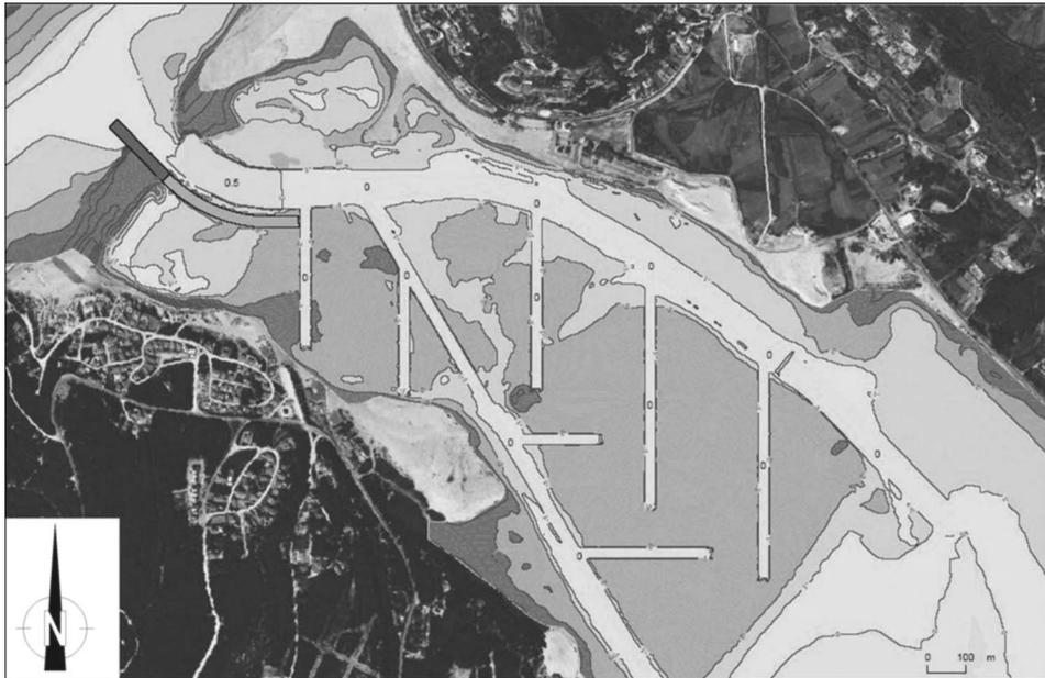
**Fig. 7.** Final solution, including the main channels, the transverse channels, and the guiding wall
