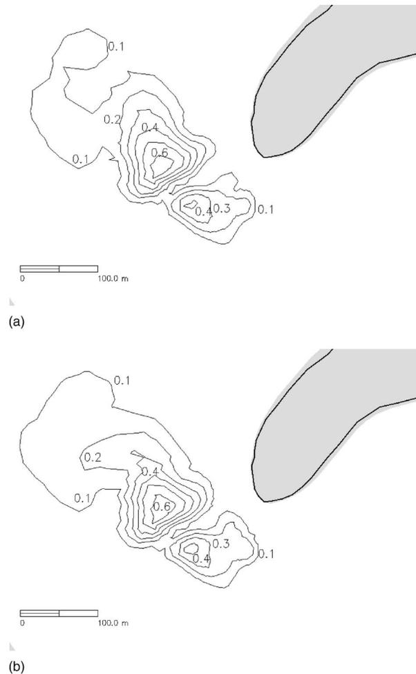
**Fig. 8.** Magnitudes of the residual sediment flux ( $\text{kg/m/s}$ ) at the inlet mouth for the configurations with: (a) the main channels alone; (b) the main and the transverse channels. All fluxes are directed seaward.
