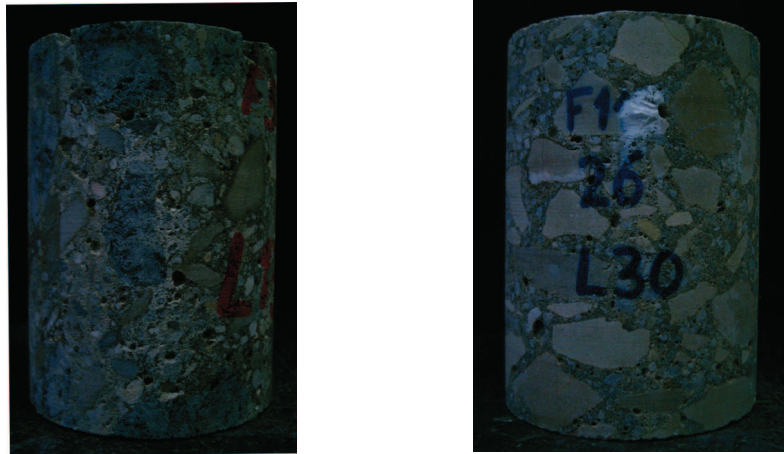
Figure 3: Concrete cores showing different characteristics in the macroscopic analysis. In the core at the left hand side voids are present close to coarse aggregate particles; the core in the centre shows damp patches around aggregate particles and higher porosity; the right hand side exhibits an exudation of alkali-silica gel (core diameter: 76 mm).
