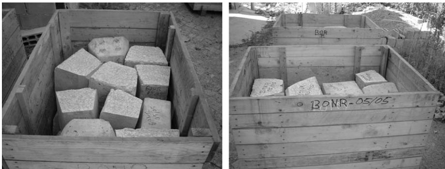
Figure 7. Storage of the concrete blocks for open-air natural weathering
