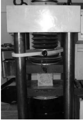
Figure 5. Hydraulic press used in the compressive strength test
