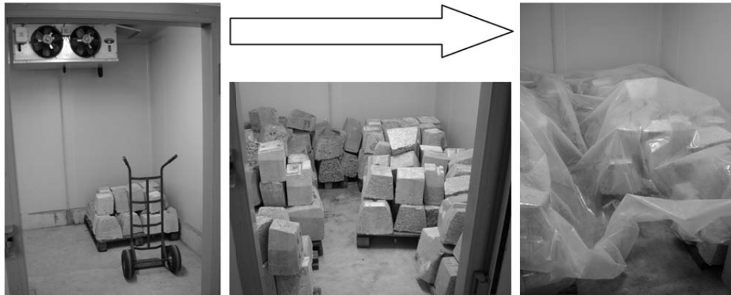
Figure 6. Storage of the concrete blocks in a climatic chamber
