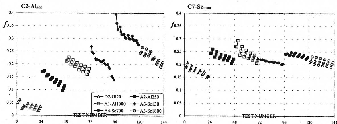
Figure 15. Friction coefficient for each test reported for the specimen C2-Al<sub>600</sub> and C7-Sc<sub>1100</sub>.
