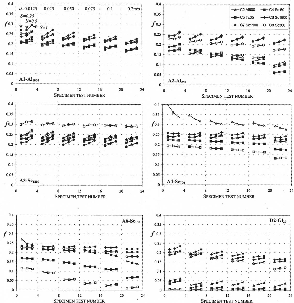
Figure 14. Friction coefficient for each test reported for every disc
