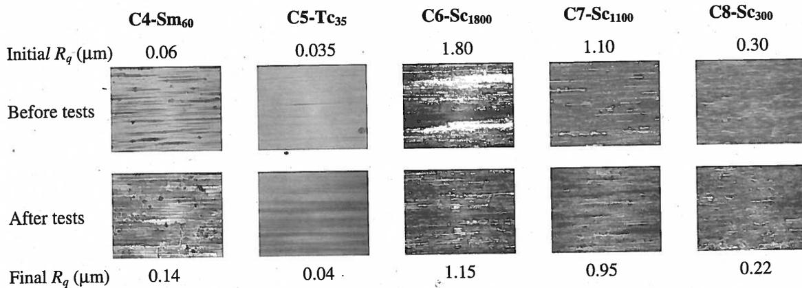
**Figure 12.** Specimens surfaces and roughness before and after the tests. Images obtained with the higher magnification (width of each image 0.81mm).
