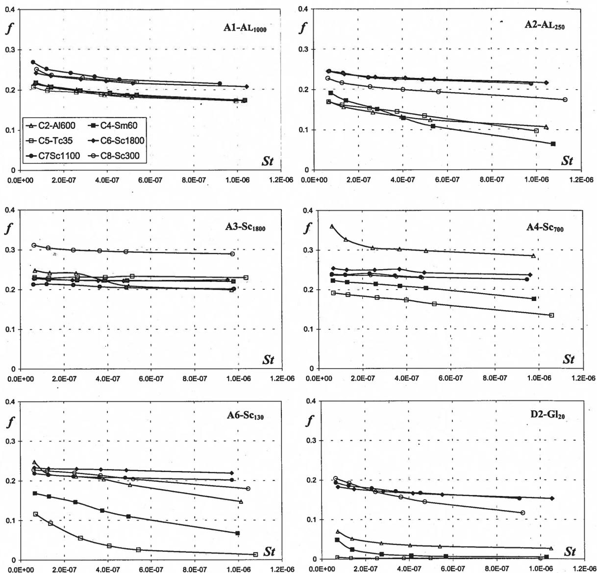
Figure 2. Friction coefficient vs. Stribeck number for the six discs,  $S=0.5$ .
