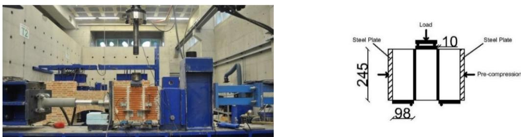
Fig. 11 | Configuration of the test setup for initial shear test and the details of the specimen (in mm)
