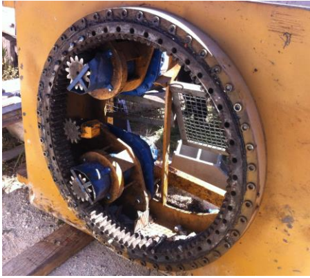
Fig. 9 | Slewing unit of the crane and its motors.
