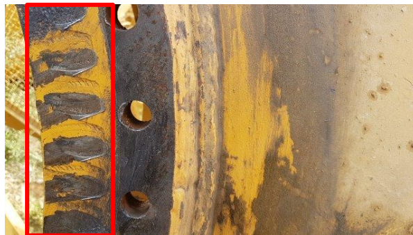
Fig. 12 | Detail of the top of the crane tower where irregular marks are visible.
