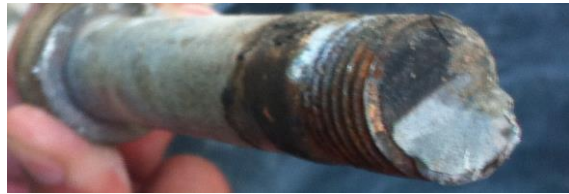
Fig. 10 | Detailed of the screw cross section evidencing brittle fracture.
