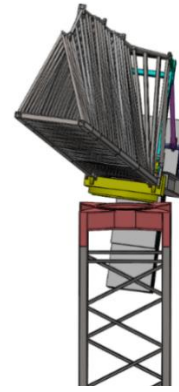
Fig. 4 | Rotation and twisting of the horizontal section of the crane.
