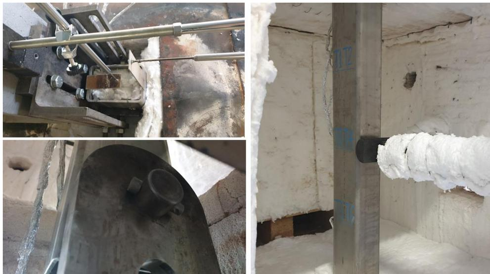
Fig. 2 | Beam inside the furnace and supporting conditions.
