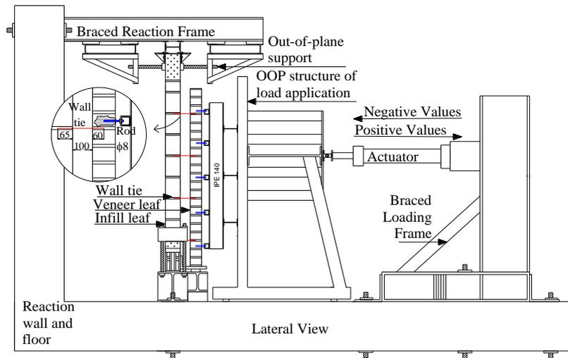
Fig. 4 | Setup scheme for out-of-plane cyclic loading
