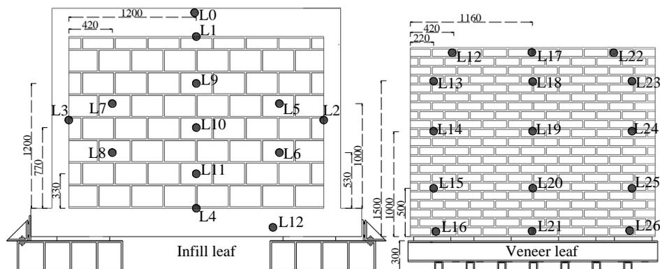
Fig. 5 | Instrumentation scheme for out-of-plane cyclic loading
