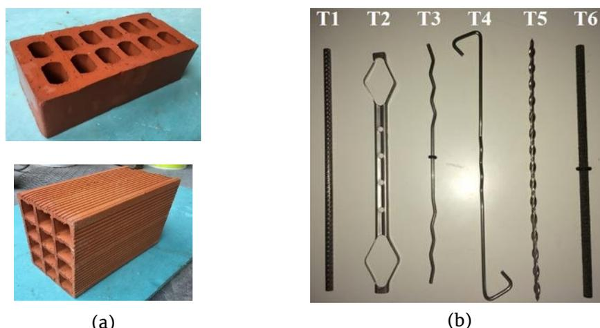
Fig. 1 | Material used in the experimental model; (a) bricks units for masonry infill and veneer Wall; (2) wall tie typologies
