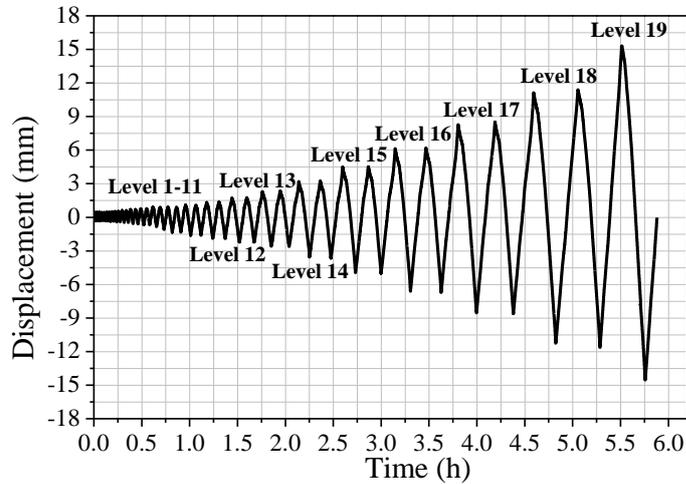
Fig. 6 | Displacement protocol for out-of-plane testing
