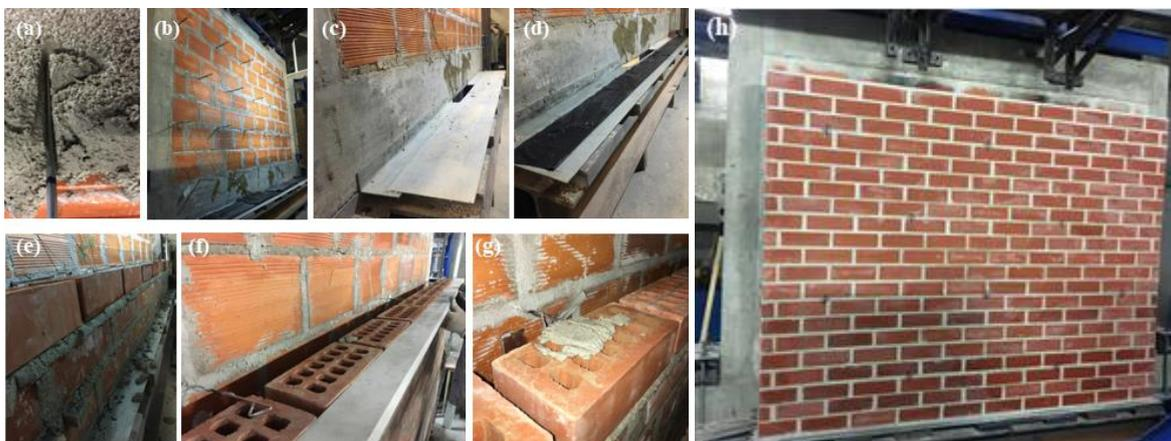
Fig. 2 | Specimen construction detailing: (a) wall tie embedment on infill leaf; (b) previous construction of infill wall; (c) shelf angle without and (d) with flashing; (e) construction of veneer wall; (f) alignment of the connectors and (g) wall tie embedment on veneer leaf (h) global view of specimen
