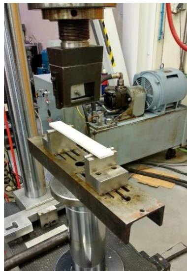
Fig. 1 | Three-point bending test setup
