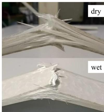
Fig. 6 | Debonding and delamination in the parts
