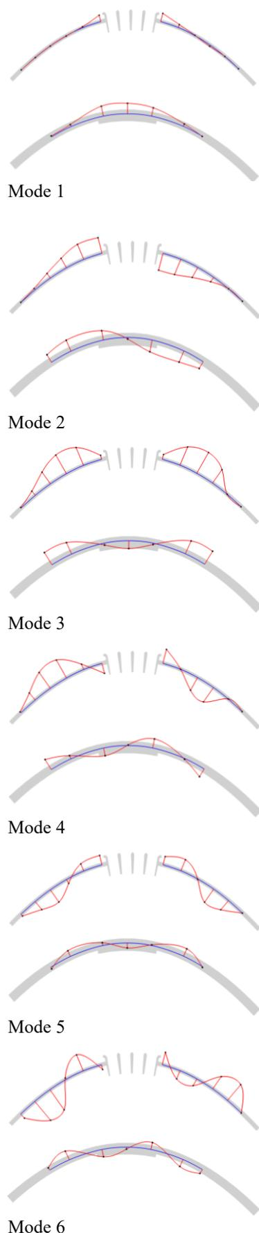
**Fig 5** - Modal configurations of the first six modes of Baixo Sabor arch dam obtained with forced vibration tests
