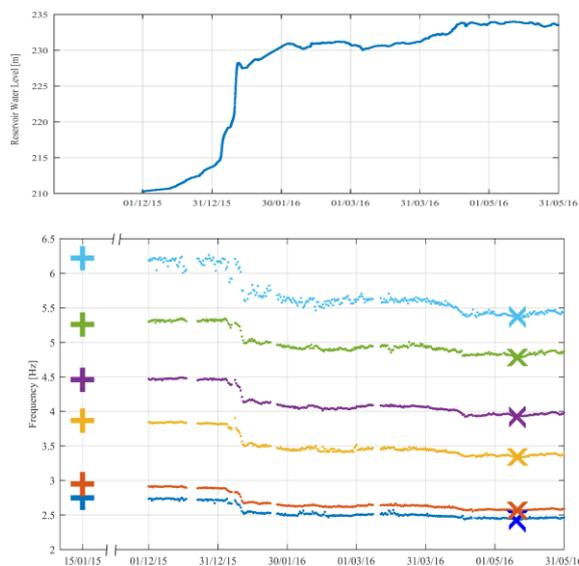
**Fig 10** - Reservoir water level evolution over time; natural frequencies evolution over time with results from forced vibration tests
