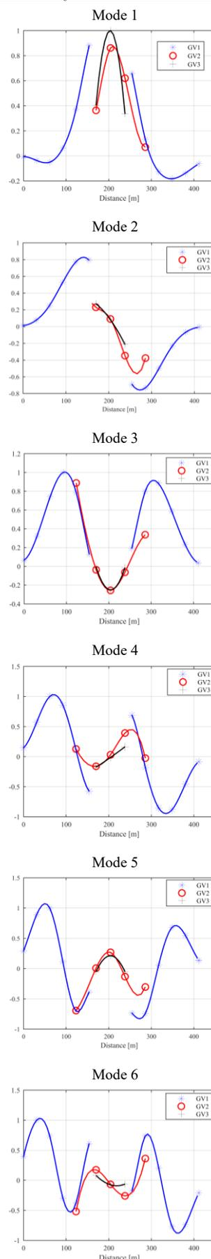
**Fig 9** - Modal configuration of the first six modes of Baixo Sabor arch dam obtained with operational modal analysis
