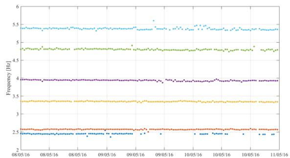
**Fig 8** - Identified natural frequencies before, during and after the second forced vibration test
