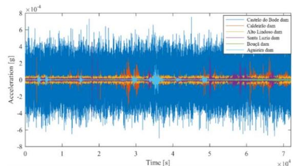
Fig 3 - Time series of accelerations collected in the whole set of tested dams
