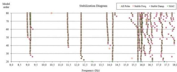
Fig 10 - Stabilization diagram obtained after the application of SSI-cov method to data from Caldeirão dam
