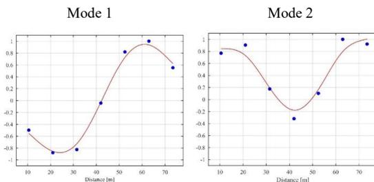
**Fig 12** - Mode shapes of the identified modes of Caldeirão dam
