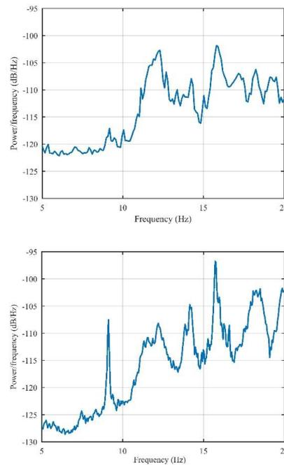
Fig 11 - Auto-spectra from time series recorded inside the upper visit gallery (top) and from time series recorded in the top viaduct (bottom)
