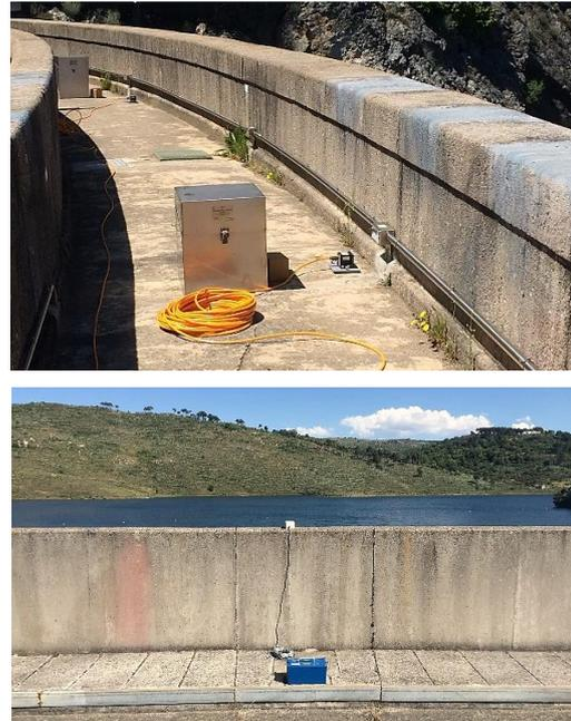
Fig 2 - Sensors positioned during tests: uniaxial accelerometer with cable (top); tri-axial recorder with GPS antenna (bottom)
