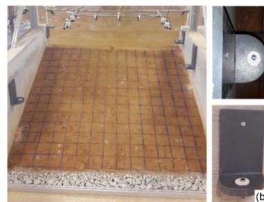
**Fig. 12** - Kinect sensor layout (a) focal positions adopted in the area scanning; (b) position of the targets with known coordinates
