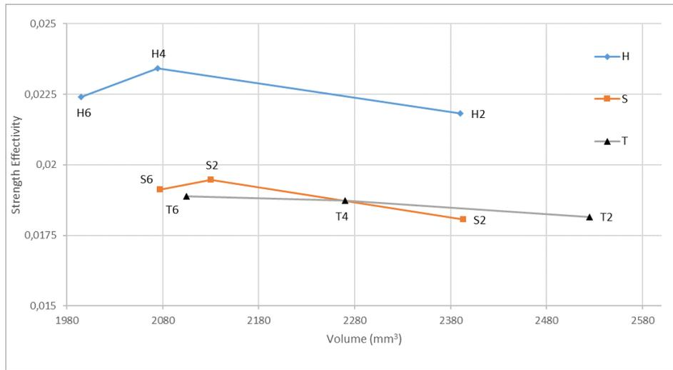
**Fig 8:** Comparison of Strength Effectivity by Volume for specimens with different inner structures
