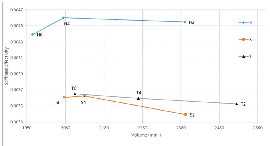
**Fig 9:** Comparison of Stiffness Effectivity by Volume for specimens with different inner structures
