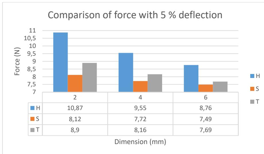
**Fig 5:** Comparison of Force with 5% deflection for specimens with different inner structures
