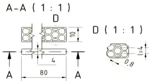
Fig 2: Specimen with hexagonal shape and 4 mm dimension of inner structure
