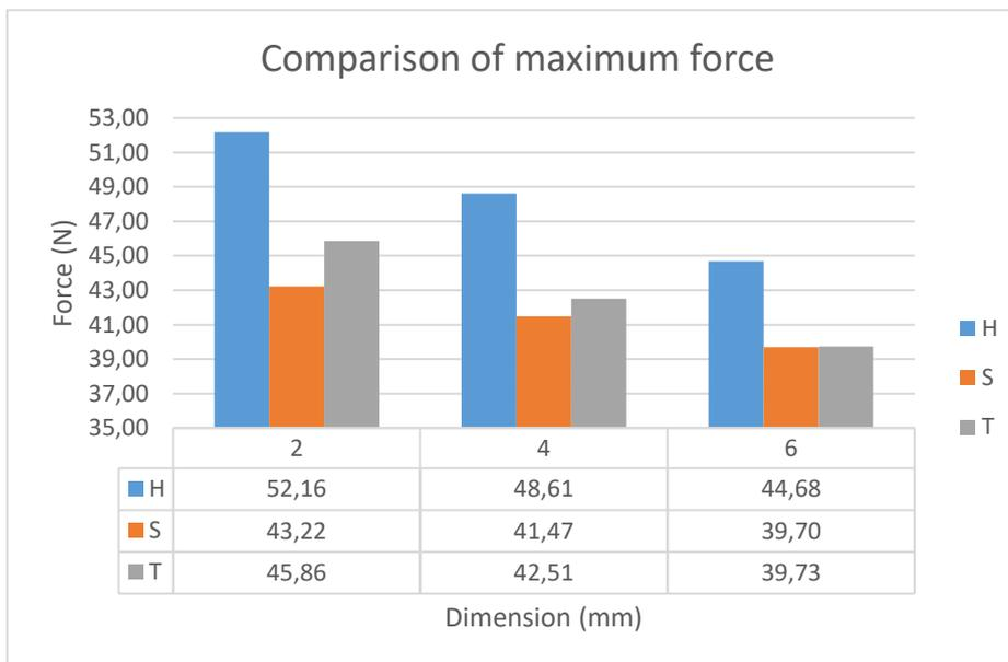
**Fig 6:** Comparison of Maximum Force for specimens with different inner structures
