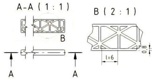
Fig 4: Specimen with triangle shape and 6 mm dimension of inner structure
