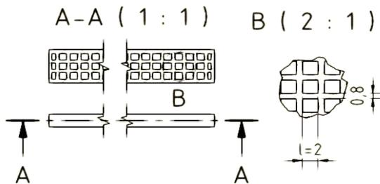
Fig 3: Specimen with square shape and 2 mm dimension of inner structure
