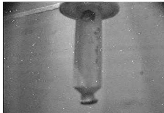
Fig. 5 - Aluminum-clad fuel element with kneaded bottom end-pin [10].
