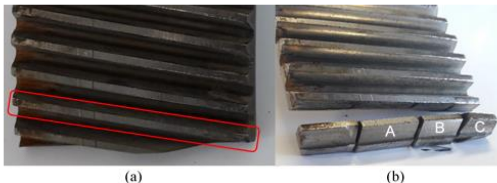
Fig 5 – Specimens cutting for teeth analysis: (a) Section of the gear teeth choose for analysis; (b) teeth A, B and C cut with a grinding wheel
