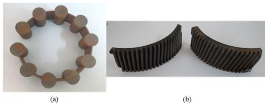
Fig 3 - (a) Samples obtained from the inner part of the helical gear; (b) teeth samples obtained for analysis
