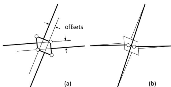
**Fig. 1** – Kinematics of joint models: (a) Krawinkler type model, (b) rotational springs attached to beams ends joint model.
