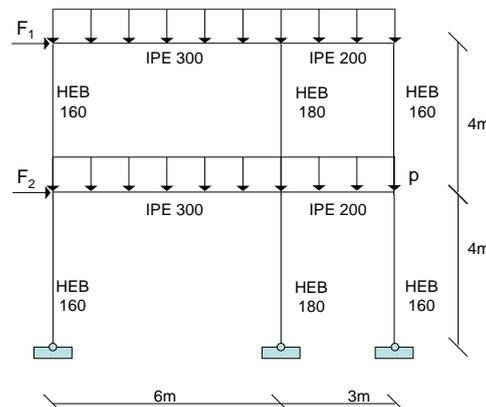
**Fig. 14** – Steel frame: dimensions, sections, loads
