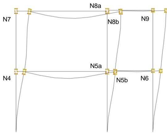
Fig. 15 – Deformed shape of steel frame and joints’ numbering.
