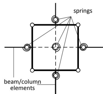
Fig. 3 – Beam-to-column joint model proposed by Altoontash (2004).
