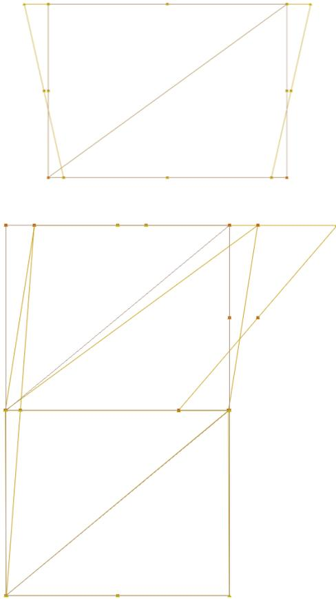
**Fig. 13** – Deformed shape for the SP model for symmetric load (top) and for the DP model for asymmetric load (bottom).
