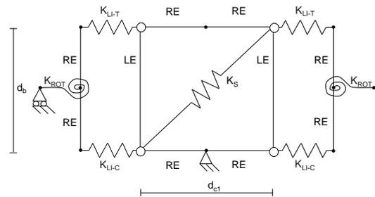
Fig. 5 – Beam-to-column joint model with beams of equal depth – single panel (SP) model.
