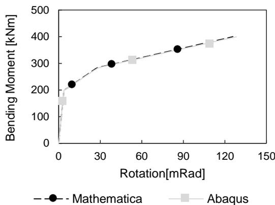
**Fig. 9** – Moment-rotation curve for right side of SP model under symmetric load condition (node 5 in Fig. 8).
