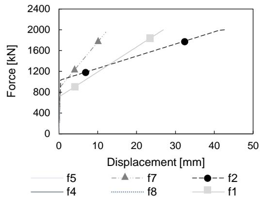
**Fig. 12** – Force-displacements relationship for tension ( $f_2, f_5$ ), compression ( $f_1, f_4$ ) and shear ( $f_7, f_8$ ) components in DP model.
