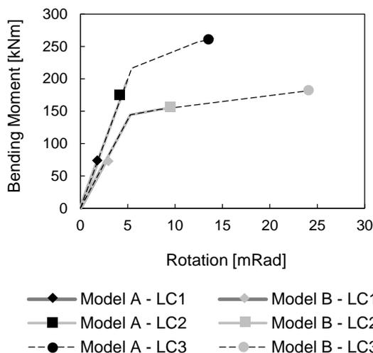
Fig. 16 – Bending moment vs. rotation of spring 3.
