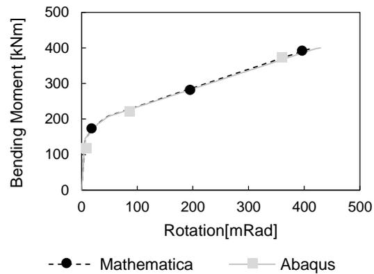
**Fig. 11** – Moment-rotation curve for right side of DP model under asymmetric load conditions (node 5 in Fig. 8).
