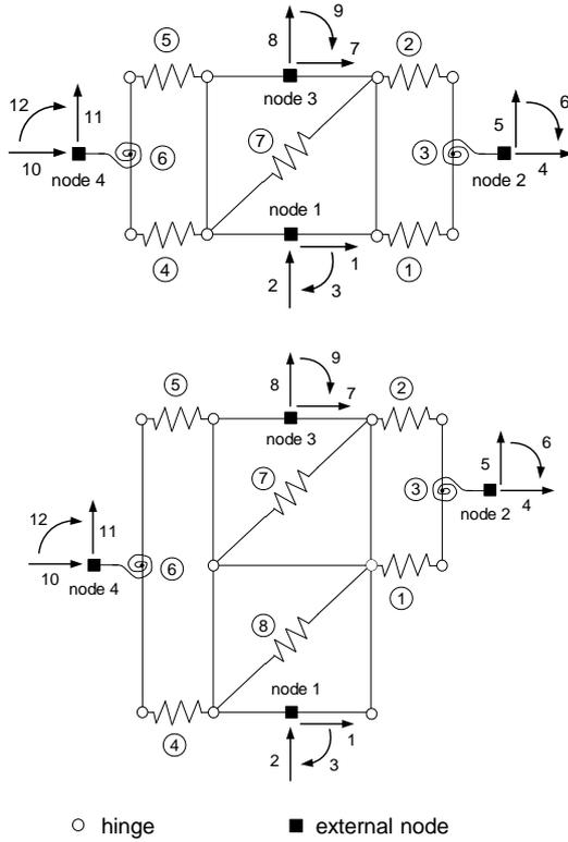
**Fig. 8** – External degrees of freedom, springs and external nodes numbering for SP model (top) and for the DP model (bottom).
