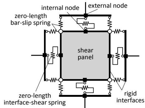
Fig. 2 – Beam-to-column joint model proposed by Lowes and Altoontash (2003).
