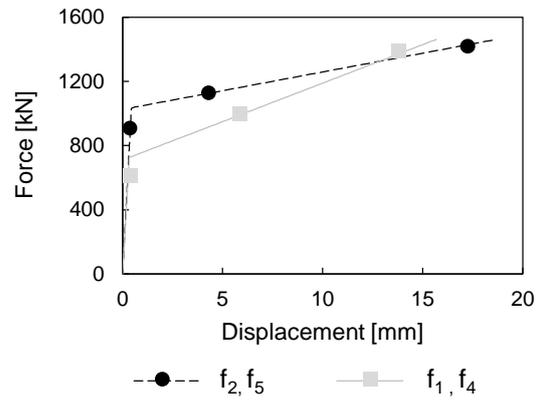
**Fig. 10** – Force-displacements relationship for tension ( $f_2, f_5$ ) and compression ( $f_1, f_4$ ) components in SP model.
