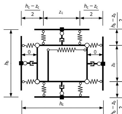
Fig. 4 – Beam-to-column joint model proposed by Costa (2013).
