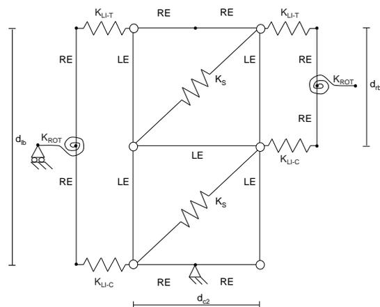
Fig. 6 – Beam-to-column joint model with beams of unequal depth – double panel (DP) model.
