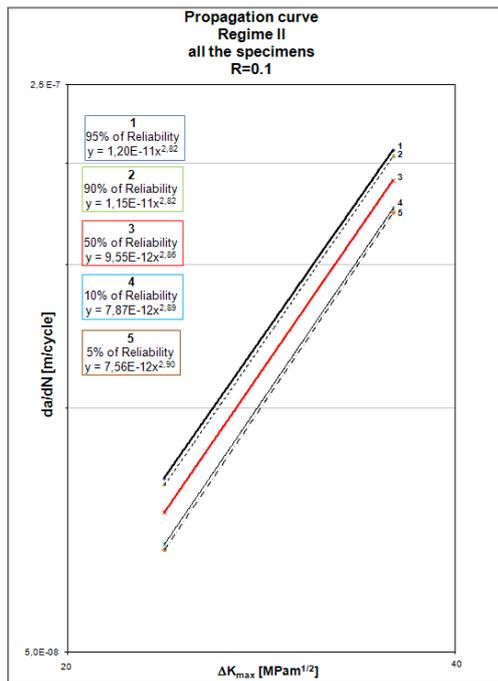
**Fig. 9** - Present the  $da/dN$  vs  $\Delta K$  curve (Paris Law), obtained from a set of raw data given for treatment of different reliability
