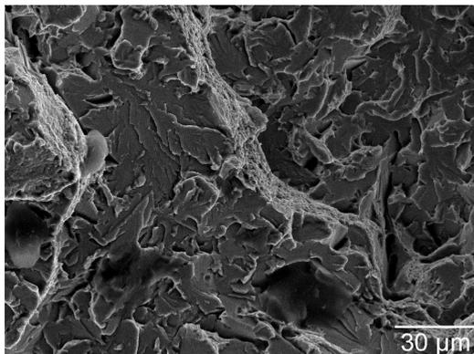
Fig. 7 - SEM fractography; high  $\Delta K=49.5 \text{ MPa}\sqrt{\text{m}}$
