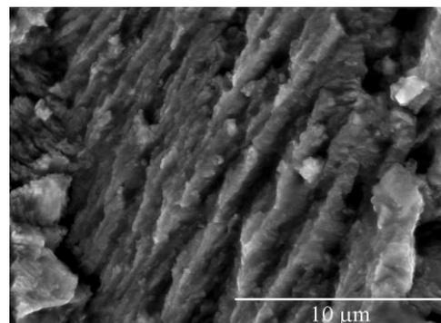
Fig. 5 - SEM fractography; near threshold,  $\Delta K=18.43$   $\text{MPa}\sqrt{\text{m}}$
