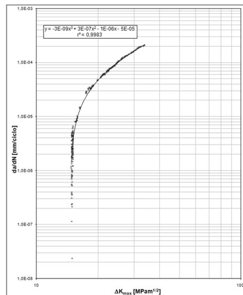
Fig. 8 - PT06 specimen propagation curve
