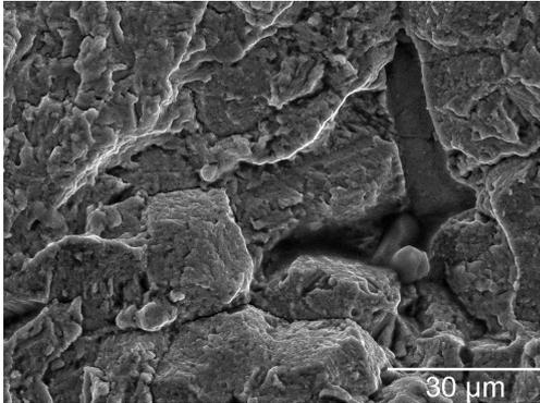
Fig. 6 - SEM fractography; Paris law regime  $\Delta K=21.31 \text{ MPa}\sqrt{\text{m}}$
