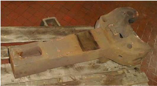
Fig. 2 – Cut zone in the railway coupling.
