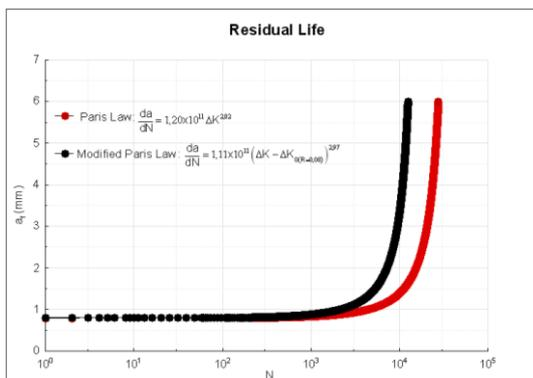
Fig. 11 -Residual life for fatigue crack propagation.
