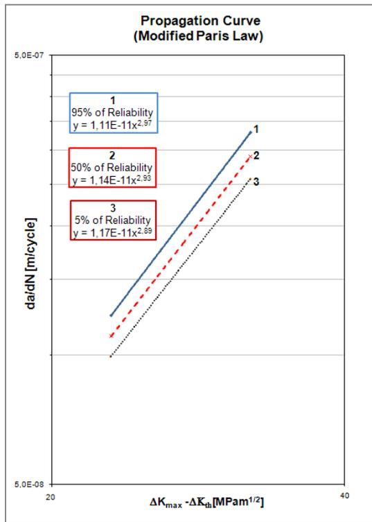
Fig. 10 - da/dN vs ΔK curve for Modified Paris Law, obtained from a set of raw data given for treatment of different reliability.
