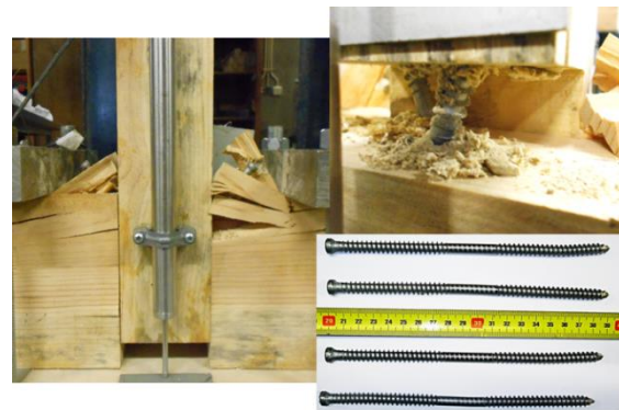
Fig. 12 – Failures observed for specimen retrofitted with self-tapping screws.
