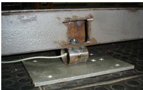
Fig. 6 - Load cell assembly on the platform.
