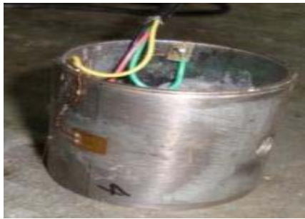
Fig. 5 - Instrumented Ring-type load cell.
