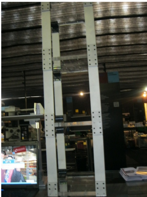
Fig 14: Three-story model at the Quanser ST-2 at FEUP [12] [13]
