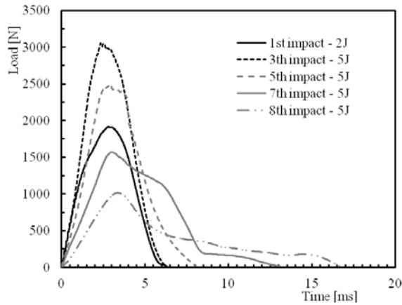
Fig. 5 Load- time curve for  $[0_2,90_2]_s$  layup.
