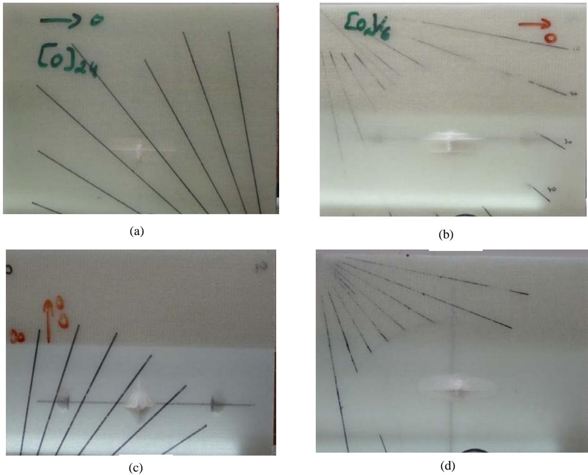
**Fig. 7** Typical damages occurred after the 6<sup>th</sup> impact for laminates: a) [0]<sub>24</sub>; b) [0]<sub>16</sub>; c) [0<sub>2</sub>,90<sub>2</sub>]<sub>s</sub>; d) [0<sub>2</sub>,90<sub>2</sub>]<sub>2s</sub>.
