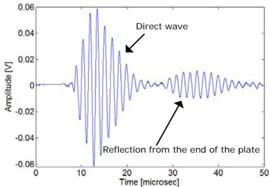
**Fig.2** Fundamental symmetrical  $S_0$  mode in the composite plate
