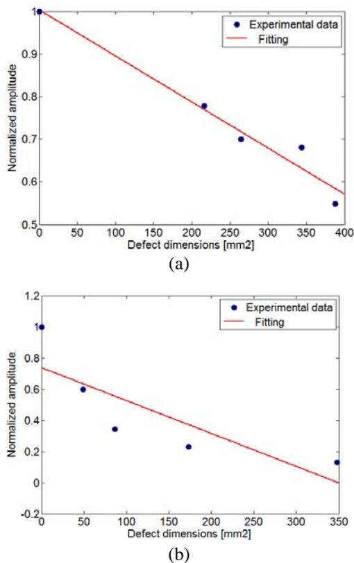
**Fig.8** Normalized signal amplitude versus defect dimensions: (a) Plate B; (b) Plate C
