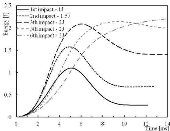
Fig. 6 Energy- time curve for  $[0_2,90_2]_s$  layup.
