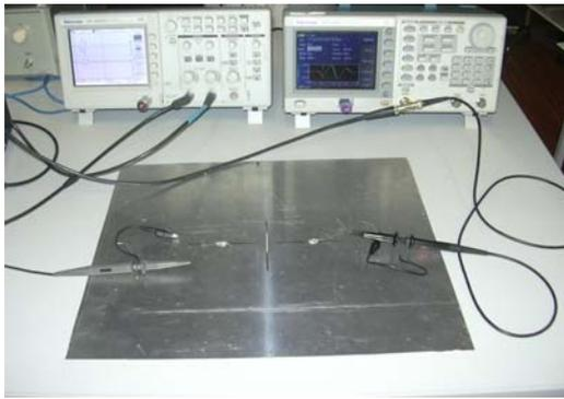
**Fig.1** Experimental setup using an aluminium plate
