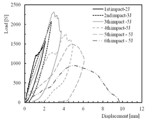
**Fig.4** Load-displacement curve for  $[0]_{16}$  composite.
