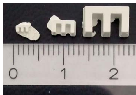
Fig.12. BST green samples obtained by gel casting process using the silicone moulds
