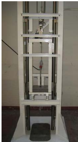
Fig. 5 – Drop weight tower.
