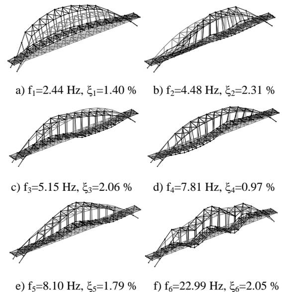
Fig 3 – Main mode shapes of Góis footbridge (AVTs).
