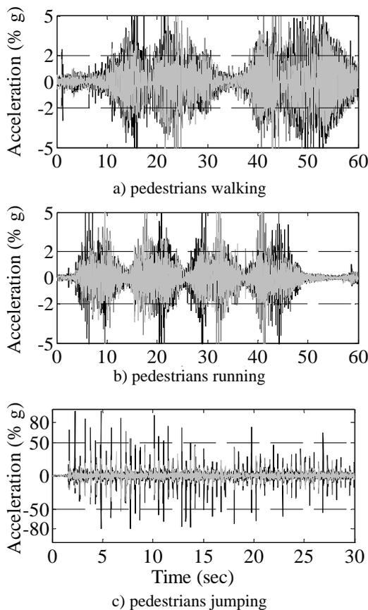
Fig 4 – Transversal acceleration response for pedestrian excitation. — — Comfort limit values.
