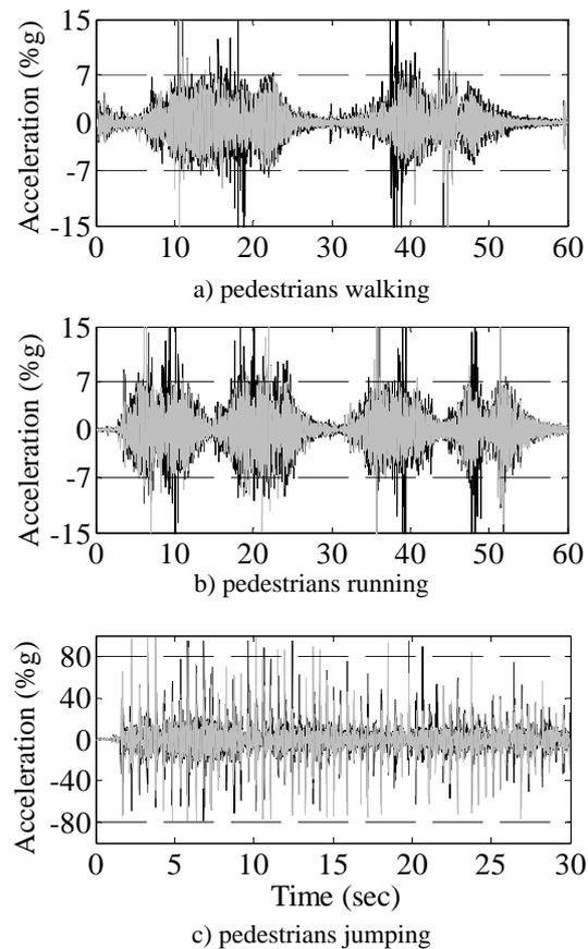
Fig 5 – Vertical acceleration response for pedestrian excitation. — — Comfort limit values.
