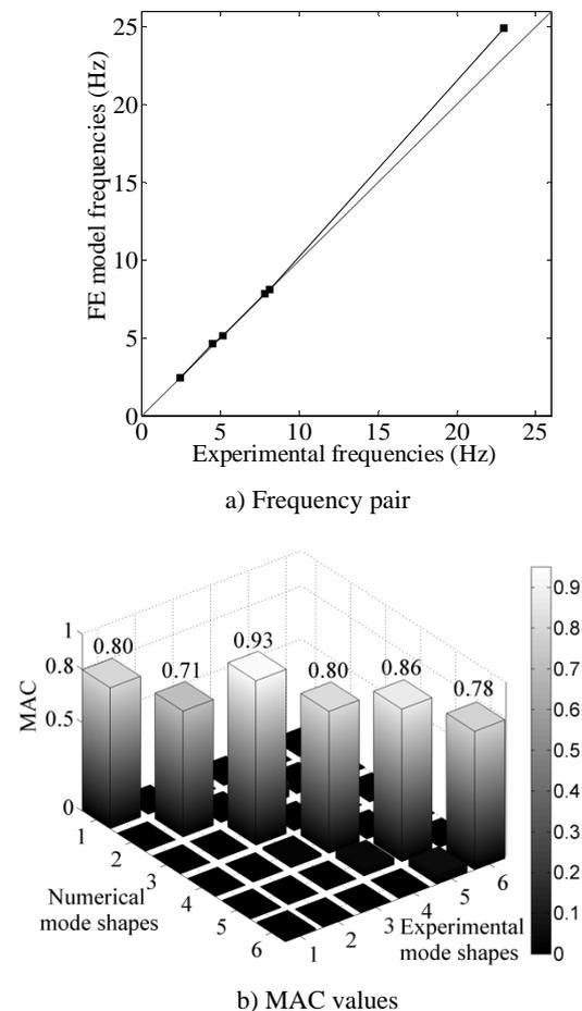
**Fig 6** – Correlation of modal parameters after the model updating procedure.
