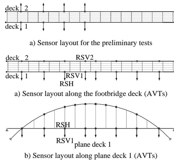
Fig 2 – Sensor layout adopted for the dynamic tests
