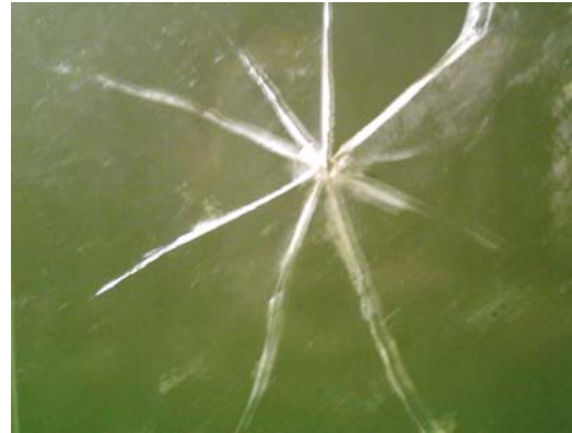
Figure2- The post impact damaged areas of a 5mm thickness glass target struck by a 7.8 mm diameter spherical projectile driven at a very low velocity.
