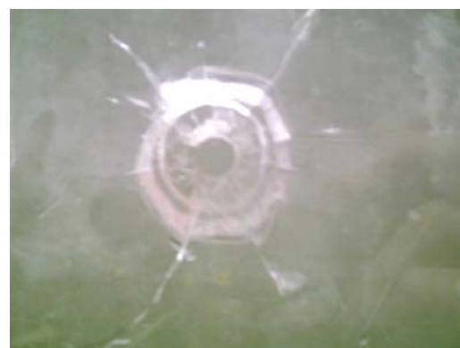
Figure3- The post impact damaged areas of a 5mm thickness Polymethylmethacrylate target struck by a 7.8 mm diameter spherical projectile driven at 250 m/s velocity.
