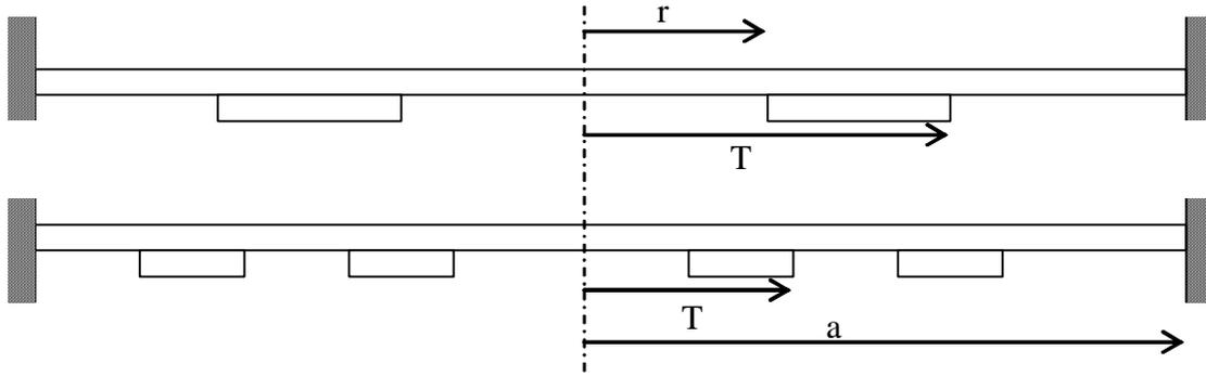
Fig 1 - a) One Stiffener Diaphragm b) Two Stiffener Diaphragm
