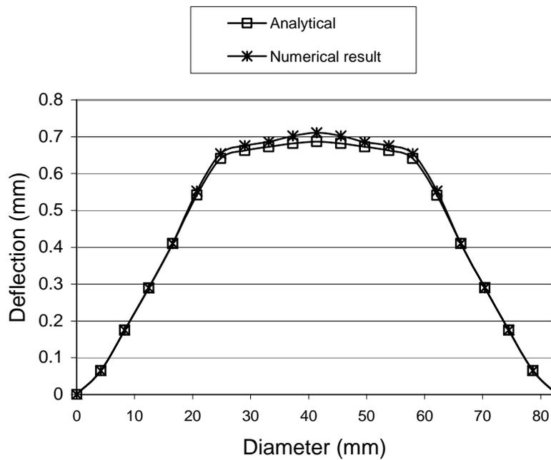
**Fig 4 -** Comparison of the results obtained by applying the recent thickness approximation technique and those obtained by the finite element method for case 3
