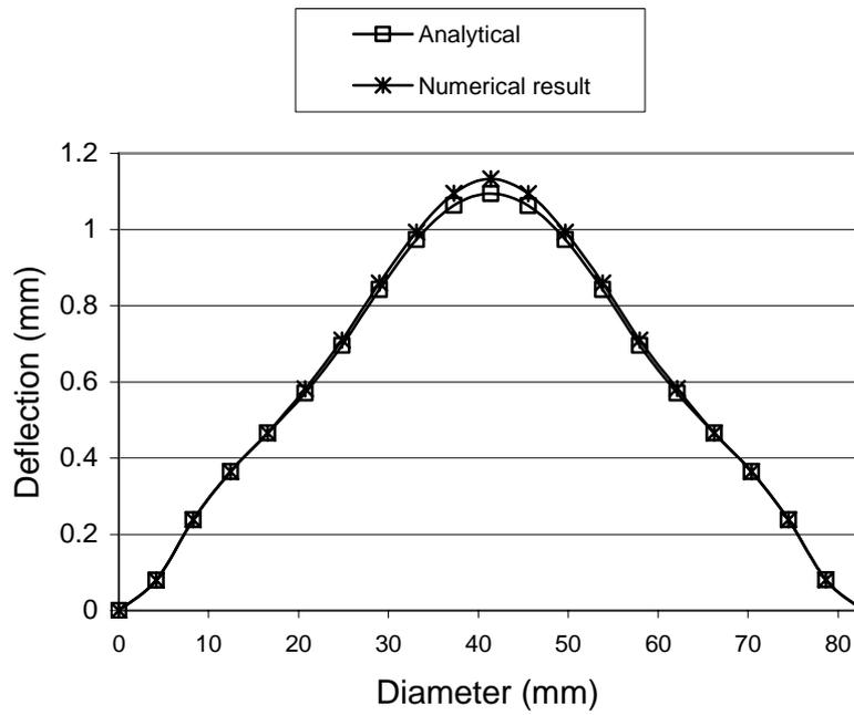
**Fig 3 -** Comparison of the results obtained by applying the recent thickness approximation technique and those obtained by the finite element method for case 2
