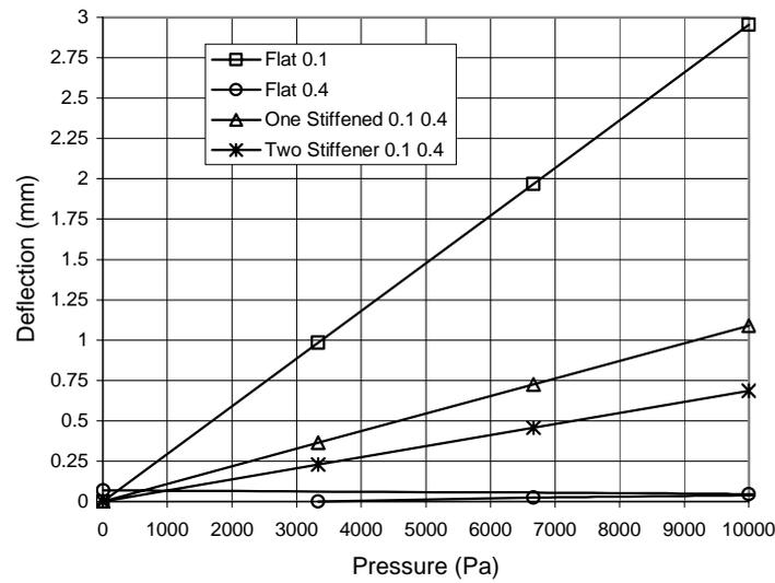
**Fig 5** - The external applied uniform pressure versus the maximum deflection at the center point of the diaphragm for all of the studied cases
