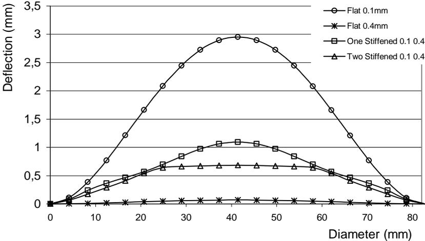
**Fig 2** - Deflection of the four different cases against radial coordinates obtained by using the analytical method
